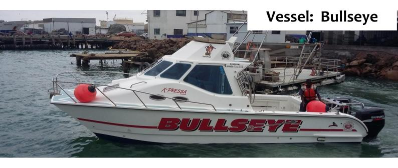
Vessel Name: Bulls Eye Type: Lee Cat Port of Registration: Walvis Bay **Registration Number:** WB 267 **Certification:** Class A Length: 9 m Draft: Approx 500mm - 600mm Deck m2: 6 Deck m3: 12 Max Speed: 30 Knots **Propulsion:** Twin 200hp, four stroke outboards Max Pax: Carrying capacity: 2,5t Safety Equipment: As per local regulation for class of vessel **Communication: VHF Radio**
